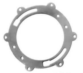
United States Patent 5.890.239 Unique screw tabs attach to wood or concrete. Plastisol coat provides corrosion protection. Slotted for 1/4" or 5/16" closet bolt. Old closet ring does not need to be present. Replaces any and all closet rings.
